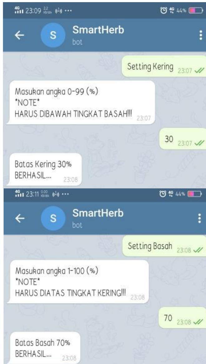
Figure 11 Dry Setting / Wet Setting
