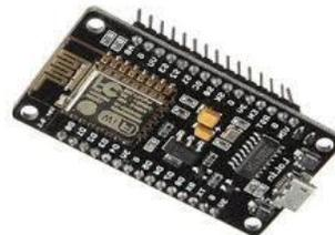
Figure 3 Node MCU ESP 8266
