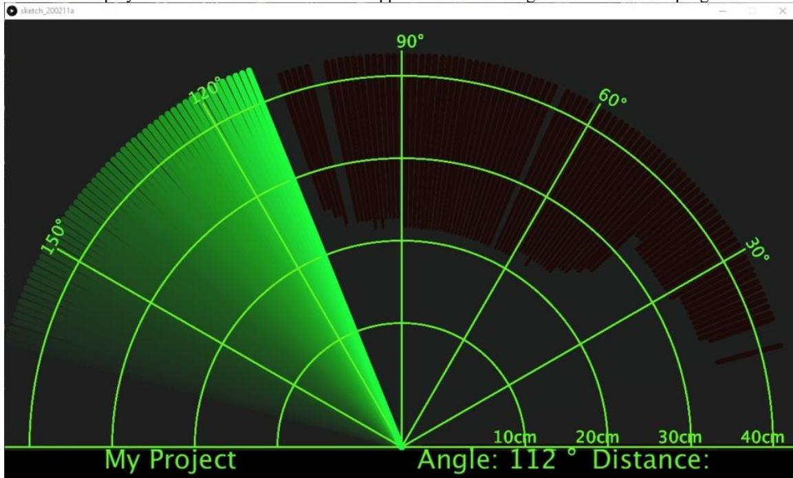
Figure 5 User Interface for Object Detection Radar with Ultrasonic Sensor Using Arduino Based on IoT on Desktop
