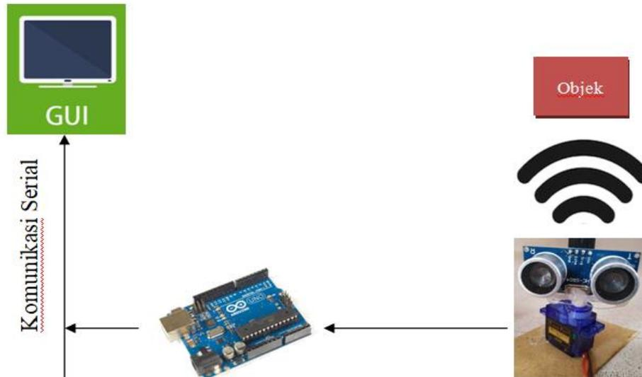
Figure 3 Schematic of Object Detection Radar Prototype Using Ultrasonic Sensor Using Arduino Based on IoT
