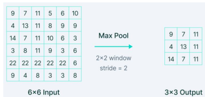
Fig. 4 Example of Max Pooling on a 6x6 Dimensional Feature Map using Stride 2
